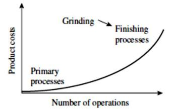
Note. The buildup of costs and value-added in product manufacture. From Principles of modern grinding technology, Elsevier, Boston MA. p.6. Copyright 2023 by Elsevier
