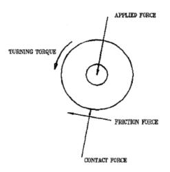
Note. Equilibrium of forces on the grinding wheel. From "Thermal analysis of the grinding process" by Gu et al. 2004, Mathematical and Computer Modelling. 39. p.993. (https://doi.org/10.1016/j.mcm2003.07.009). Copyright 2023 by the Journal of Mathematical and Computer Modelling
