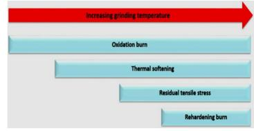
**Note.** A graphical representation of the role of temperature on the occurrence of thermal damages. From "A comprehensive review on the grinding process: Advancements, applications and challenges" by K. Kishore et al., 2022, Journal of Mechanical Engineering Science, 236(22), p.5. (https://doi.org/10.1177/09544062221110782). Copyright 2023 by the Journal of Mechanical Engineering Science.
