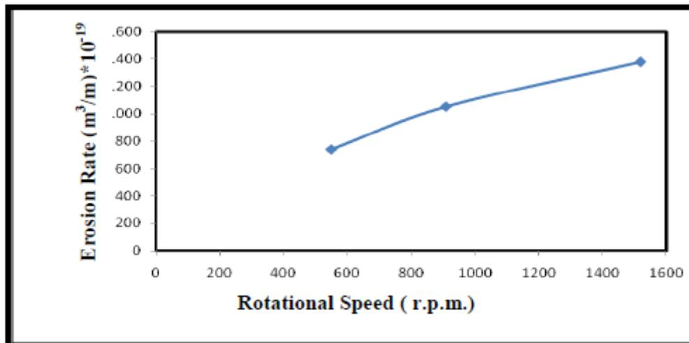
Figure (10): Shows the variation of the erosion rate with model rotation speed in the presence of barriers (impact angle  $30^\circ$  and concentration 20 wt.%).
