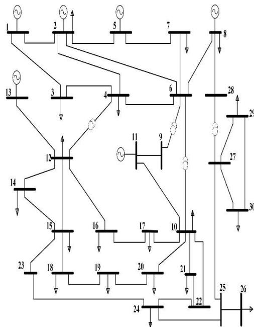
Fig. 3 Single line diagram of IEEE 30-bus system
