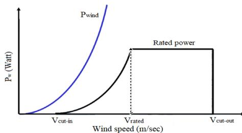
Fig. 1 Wind turbine output power curve
