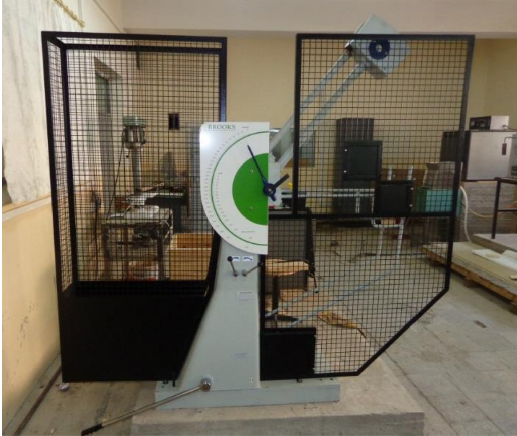
Figure 9: (a) Impact resistance test apparatus, sample
