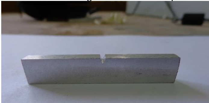
Figure 7: Standard Impact Test Sample
