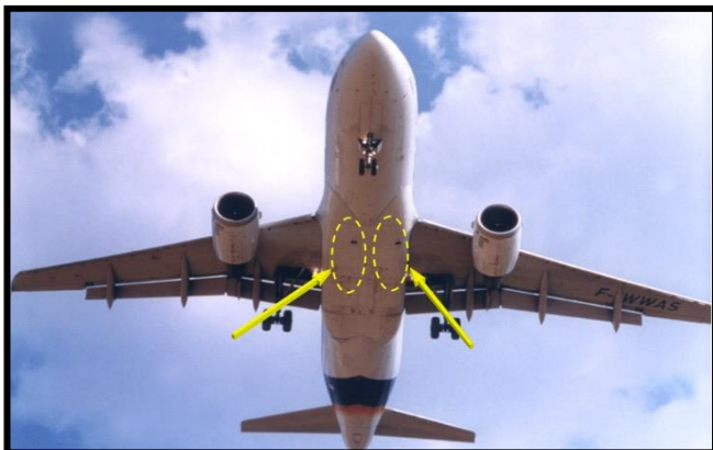
Figure(2-3) : two air conditioning packs located in the wing root area forward of landing gear bay
