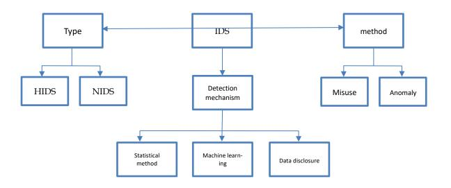
Figure (1) Overview of the IDS intrusion detection system
