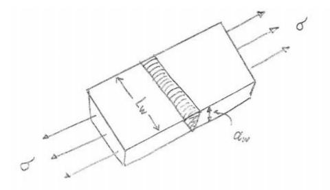
calculate which weld can sustain a load force of 360 KN, the tested weld or non-tested weld of SF=1.2 and SF=2 respectively?
